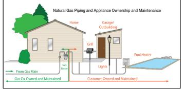
METER ACCESS: The natural gas meter and shutoff valve at your property must always remain unobstructed. Building a deck over the meter, boxing the meter in with material, planting shrubbery too close, back filling, fencing, and locking gates will restrict access to the gas meter. Restricting access can cause delays in an emergency and during meter reading.
